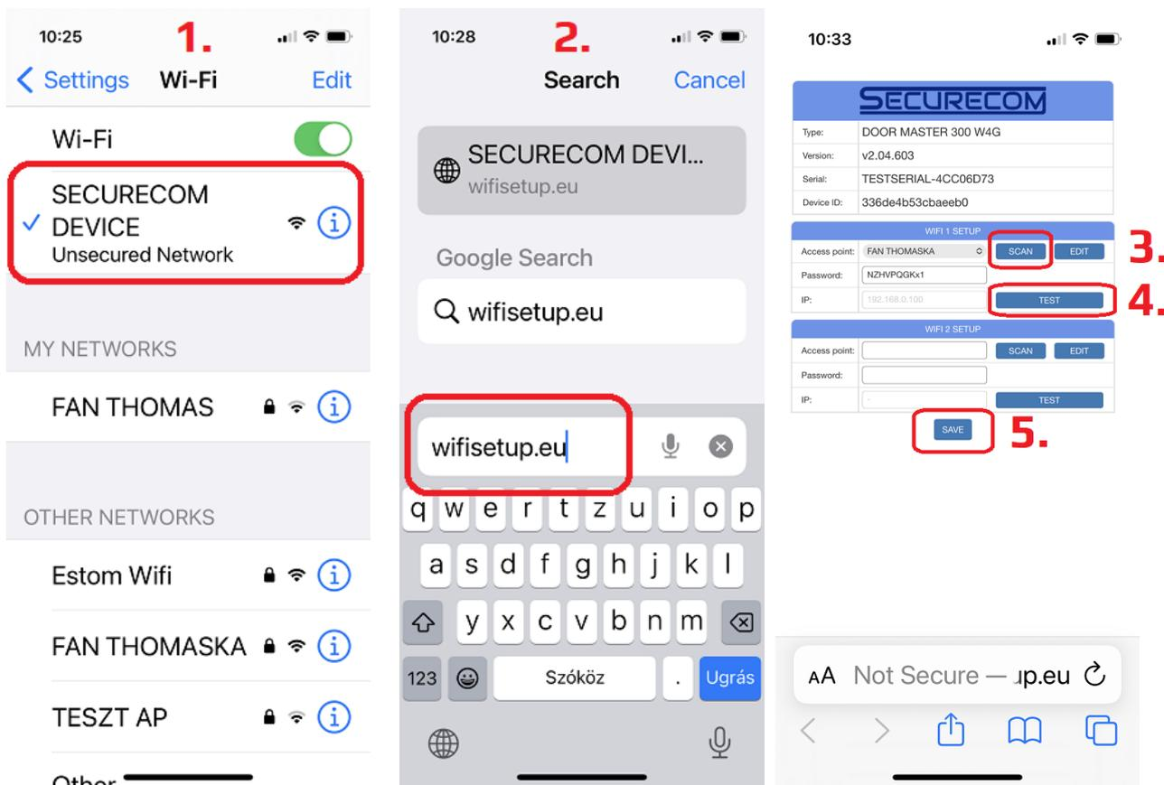
On the DP Door 300 W4G website, you can set up 2 different WIFI router connections by entering the network and password of your choice. The WIFI networks are back-up for each other, i.e. if the Internet connection on the WIFI1 network is lost, it will switch to WIFI2 and vice versa.
