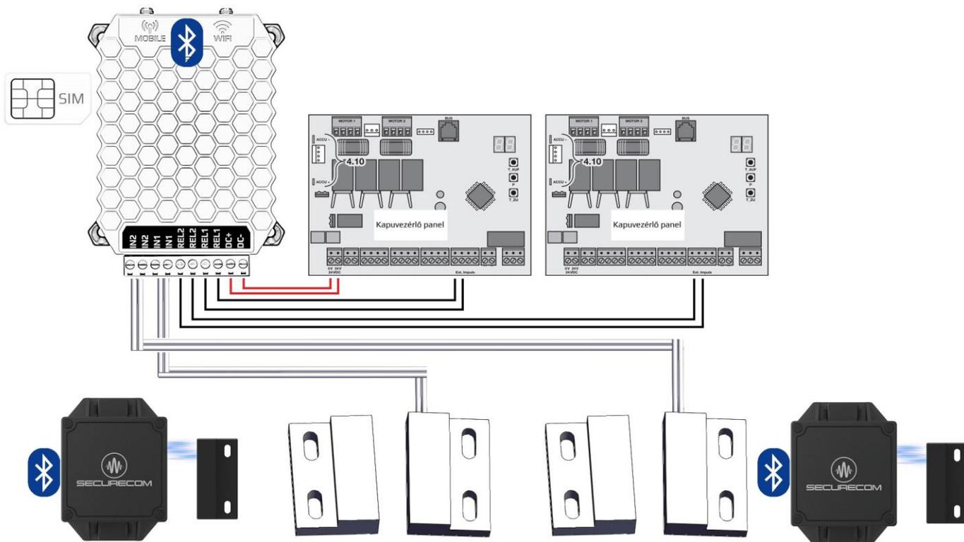
The figure shows the possible connection options for up to 2 different gate controllers. In this case, the unit is powered by only one of the gate controllers or from an external power supply. The relays trigger the opening or closing of the gate potential-free. Monitoring of the gate position (open or closed) can be done by wired or wireless SECURECOM DM-RF opening sensor.
